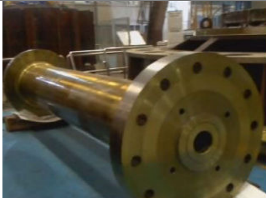
E&M works - Turbine shaft U1 & U2 - Machining completed
