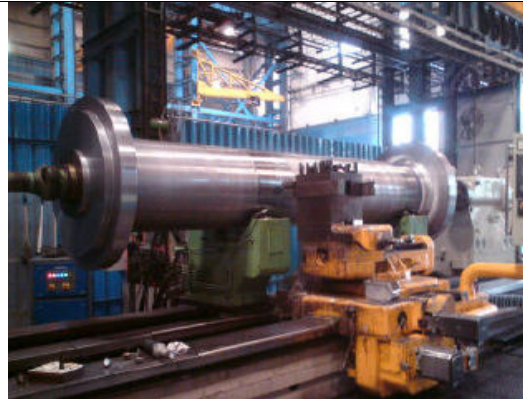
E&M works - Turbine shaft U1 & U2 - Machining completed
